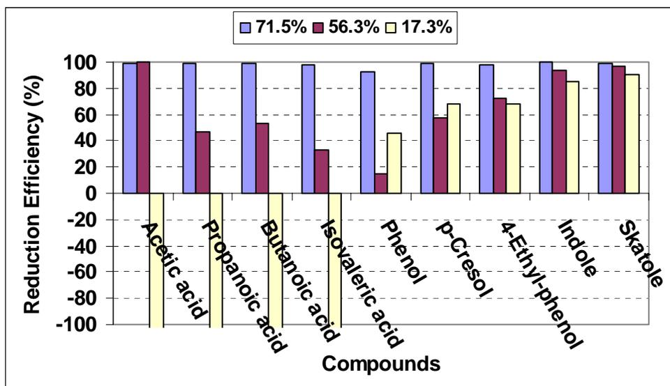
Figure 7. Reduction efficiency at different media moisture content.
