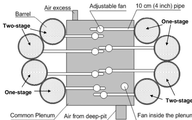
Figure 1b. The layout of the biofilter testing laboratory.
