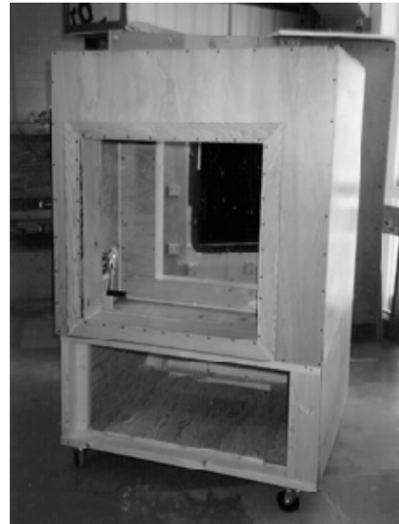
Figure 2. Sidewall test section developed for curtain infiltration study (view as seen by wind tunnel exit).
