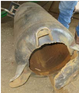
Compressed air tank with exploded bottom that was weakened by rusting.
