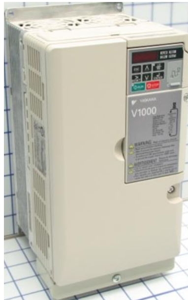
Figure A-8. Yaskawa V1000 VFD used for controlling the motion in tilting the flume.
