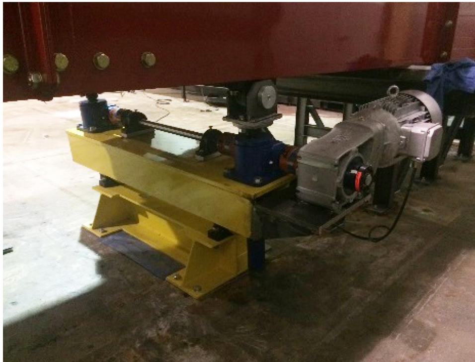
Figure A-6. Tilting actuator for raising and lowering the flume.
