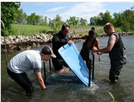
REU field trip to install seepage meters on Deer Lake, Itasca County, Minnesota
