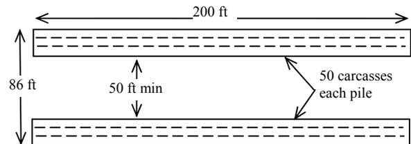
Figure 2. Example composting site dimensions for 100 cattle carcasses in two parallel windrows.
